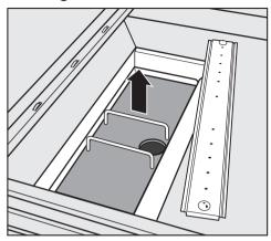
Remove the flat filter and clean if necessary.
